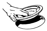
Hold the surface unit as level as possible with the terminal just started into the receptacle.
