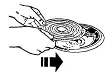
4. When the terminal is pushed into the receptacle as far as it will go, push down the edge of the surface unit opposite the receptacle. The element hold-down clip will keep the surface unit from moving around.
