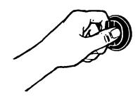
Line up openings in the reflector bowl with the surface unit receptacle and the element holddown clip.
